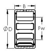
NK73/25 Bearing 2D drawings and 3D CAD models
